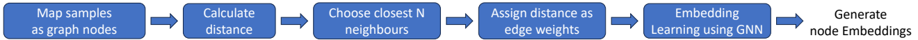
Fig. 2: Pipeline of our graph-based anomaly classification method: we map each sample as a node of a graph, calculate pairwise distances between nodes, connect each node to their nearest N neighbors with an edge-weighted by their distance, then learn and create node embeddings using GNN.
